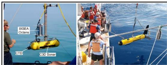
**Figure 1.** The C3D system - deployed in towfish or pole mount. DRTO survey used the pole mount.
