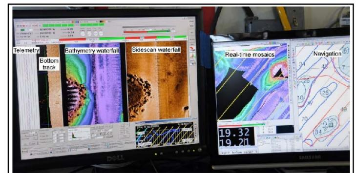
**Figure 4.** Shipboard GeoDAS acquisition and navigation.
