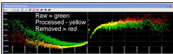
**Figure 2.** Typical bathymetric data density for 200m swath showing 10 pings.
